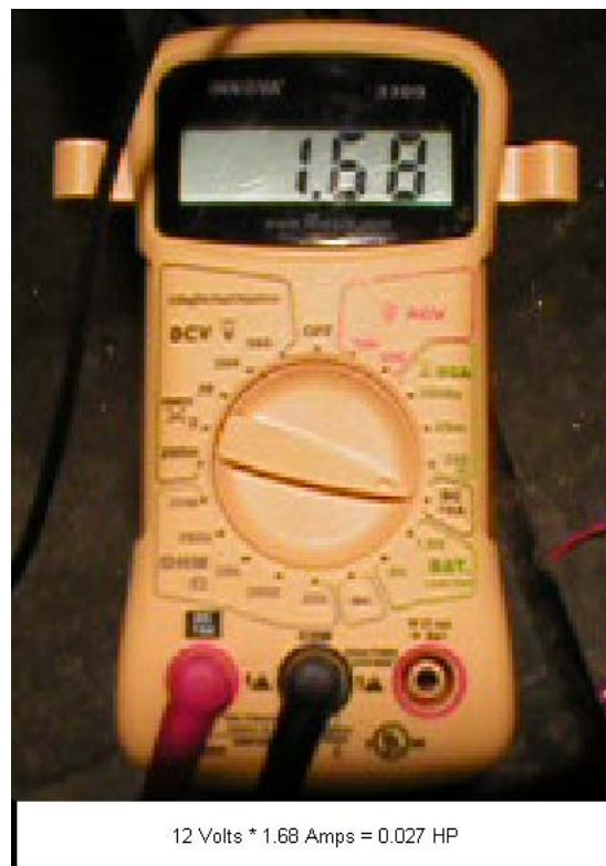
Figure 19. Linear Actuator Power Consumption
